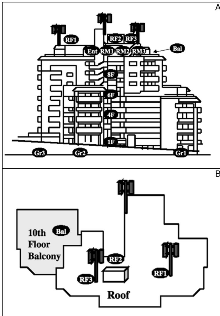
Figures 3A and 3B: Measurement points used to assess the RF-EMFs emitted from the base station on 24<sup>th</sup> December 2008; elevation view (A) and plan view (B). For an explanation of the abbreviations used refer to Table 1.
